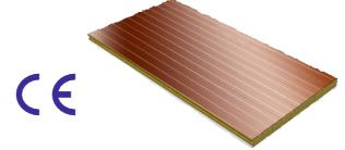
'POLAR' thermal insulation wall panel, with a visible fastening system, with (upper and lower) sides made of (PES, PVDF..) galvanised steel sheets with galvanic protection, and with a 80 mm thick stone wool core.
